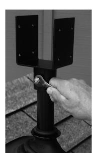
9 Secure the Saddle with the <sup>3</sup>/8" bolt, flat washer and nut (included). After tightening, there will be a small amount of play with the Saddle on the Riser, which is acceptable.
